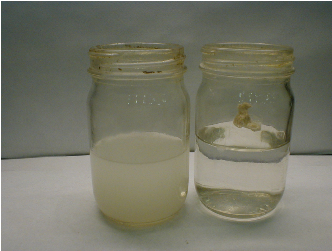
Figure 4. Fast 50 ml hand mixed jar testing with dual high molecular weight flocculants.
